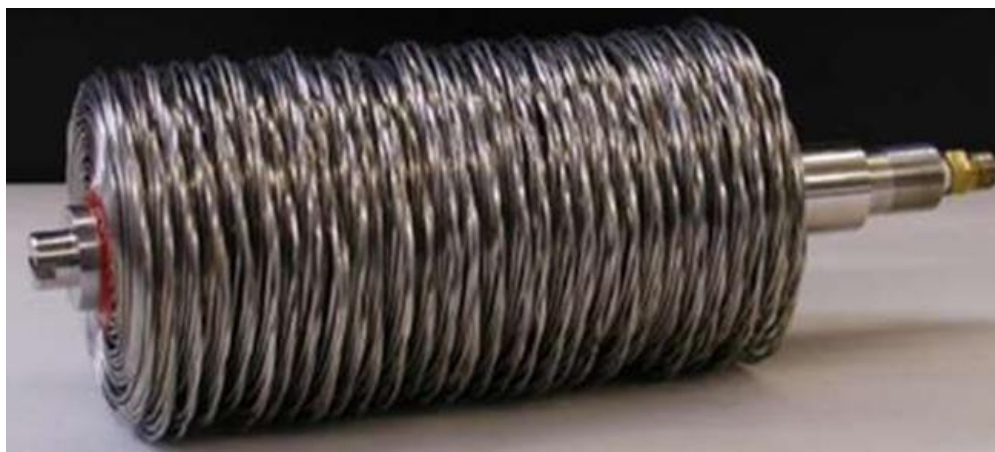
Figure 10. Metal hydride compressor.
